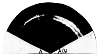
Fig. 2.—A contact print of a sector of a circular paper chromatogram of adenine and adenine hydrolysates taken in the ultraviolet using a chlorine filter. A Adenine, A(h) Adenine hydrolysate.
